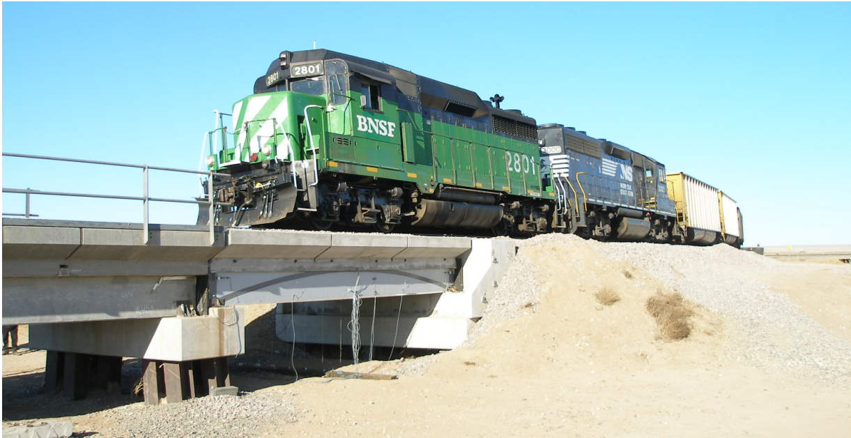
Figure 2.1: Test train crossing 30-foot prototype HCB span at TTCI Pueblo, CO, test facility
