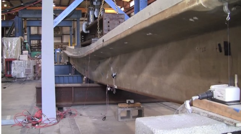
Figure 1.1. Tension field action in laboratory (Courtesy of Virginia Tech)
