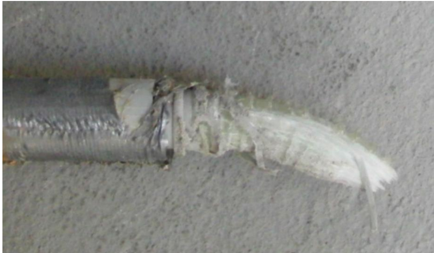
Figure 6: Failure of a bent bar with bonding
