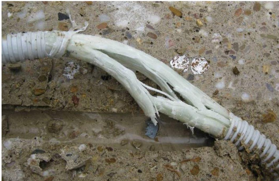
Figure 7: Failure of a bent bar without bonding
