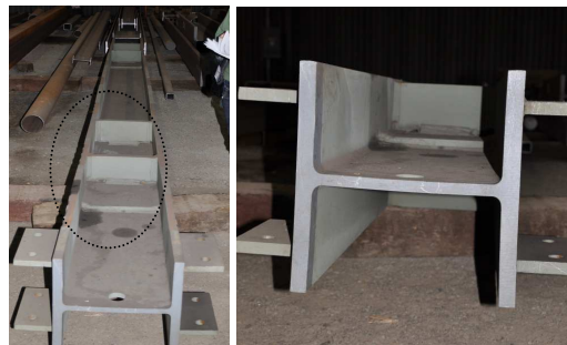
Figure 1: Prequalified connection in high strength (65 ksi / 450 MPa) W-Shape
