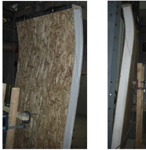
Figure 3. Views of deformed shape of wall W8
