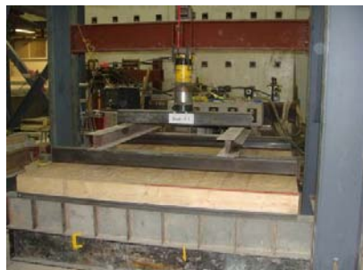
Figure 10. View of specimen SF-1 before testing
