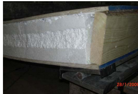
Figure 9. View of the horizontal shear failure at the interface between the foam and top OSB in model WS19
