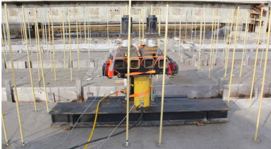
Figure 2. Front view of the test setup for double bars
