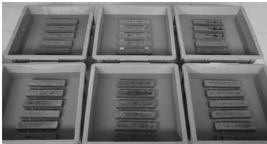
Figure 4: Immersion of concrete specimen in corrosive solution
