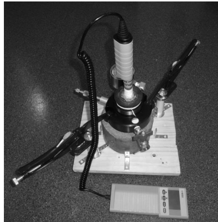
Figure 1: Specimen surface relative humidity measurement
