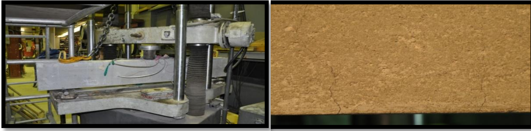
Figure 5: Pre-cracking by Tinius Olsen Jack (left). One mm width pre-loading cracks before environmental exposure (Right)
