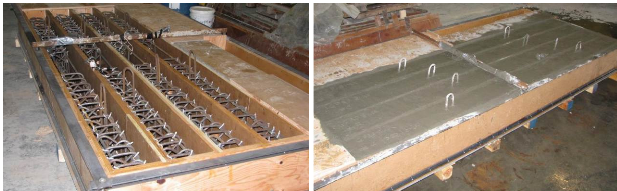
Figure 3: Fabrication of beam specimens
