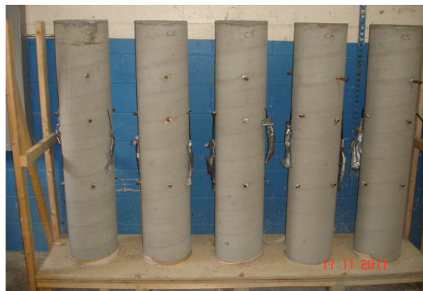
Figure 2: Fabrication and preparation the column specimens
