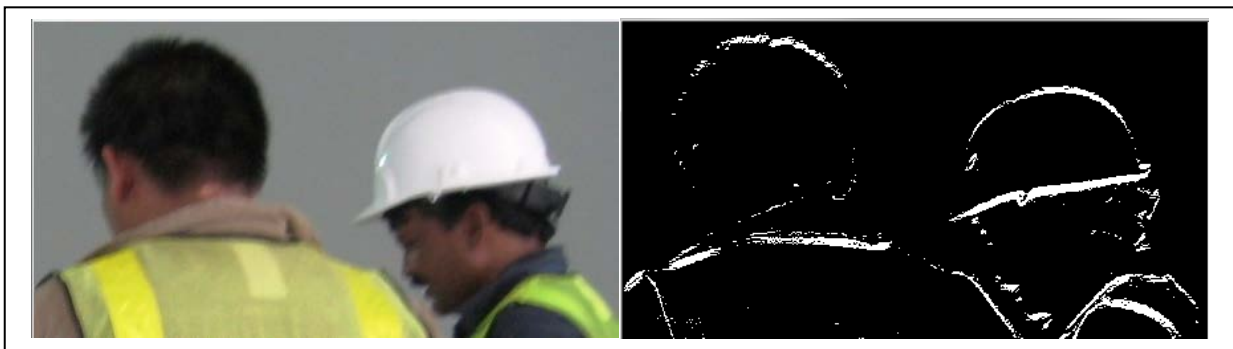
Figure 6: An RGB photo of two workers (left) one with no hard hat and the other with a hard hat. The program can distinguish the VOP of each worker as being with and without a hard hat.
