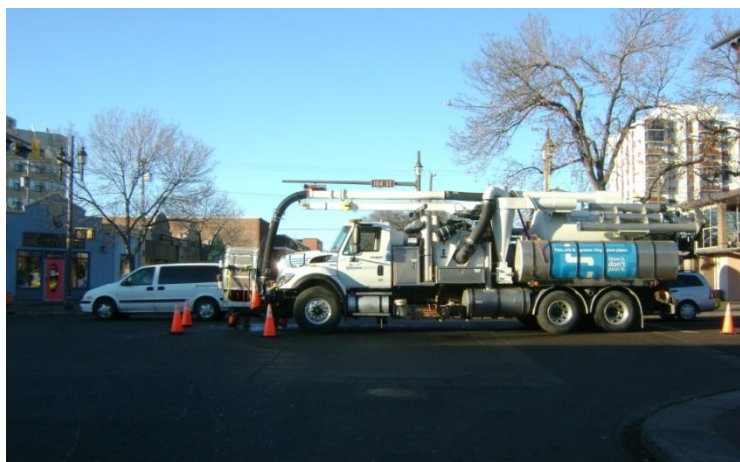
Figure 1: PM vehicle (combo unit) performing high-pressure flushing
