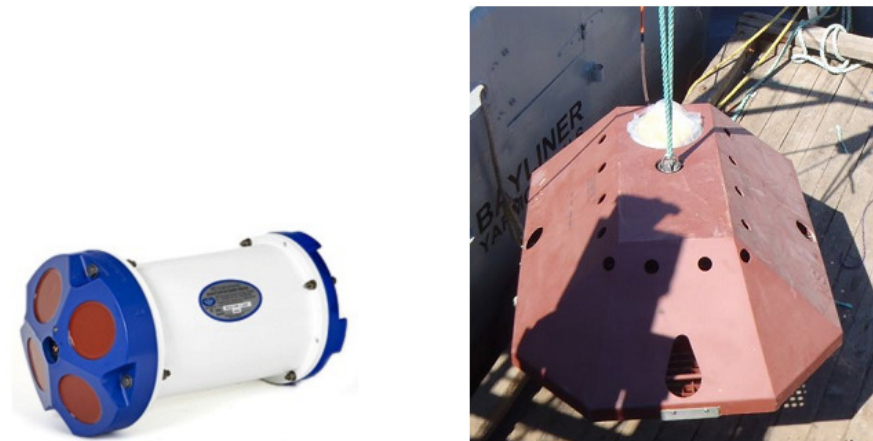
Figure 3: Workhorse Sentinel in standalone (left), and bottom-mounted (right) configurations (TRDI 2011)
